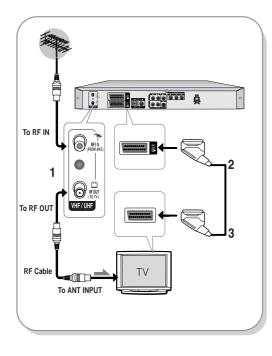
The RF cable connection of this DVD Recorder sends only signals of TV. You must connect SCART cable or Audio/Video cables to watch a signal from your DVD Recorder.
